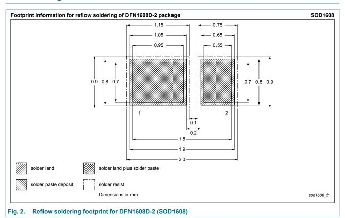
plastic, leadless ultra small plastic package; 2 terminals; 0.94 mm pitch; 1.6 mm x 0.8 mm x 0.37 mm body
