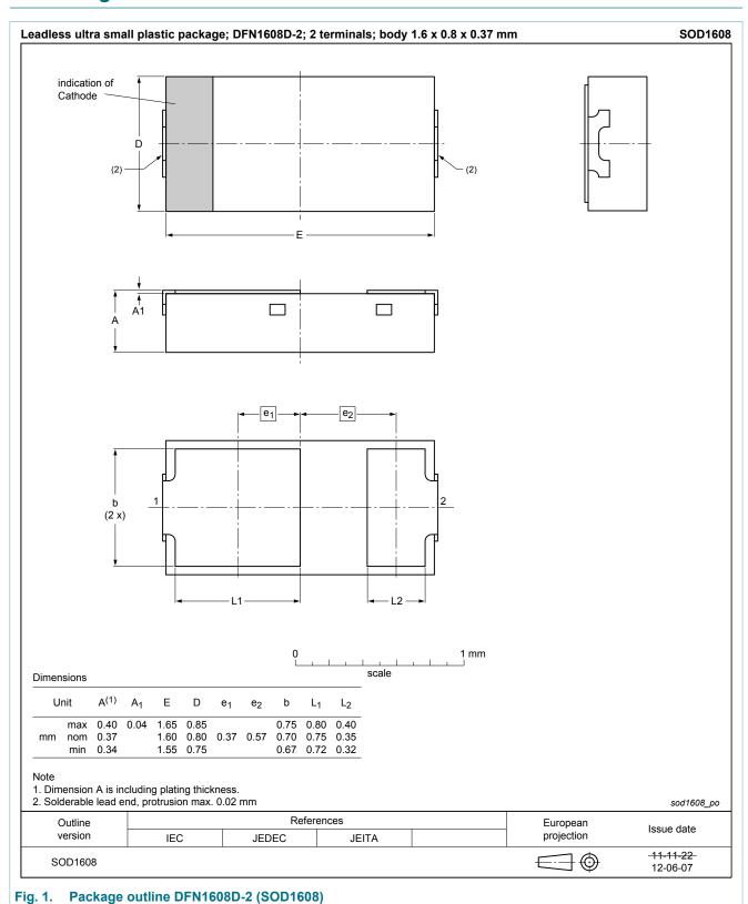
plastic, leadless ultra small plastic package; 2 terminals; 0.94 mm pitch; 1.6 mm x 0.8 mm x 0.37 mm body
